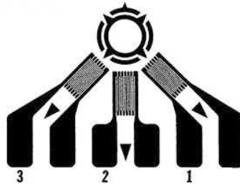
Figure 3.12: Hole drilling rosette.
